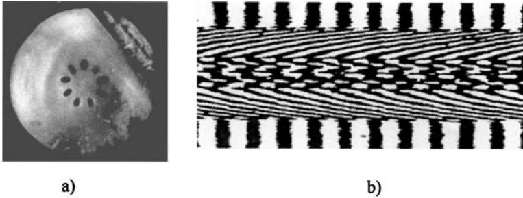
**FIGURE 4** a) Photography of a nine-elliptical core optical fiber cross-section; photo enlarg. 144x; b) Interferogram of nine-elliptical core fiber, exposed for the investigation;  $n_L = 1.591$  and  $\lambda = 632.8$  nm.
