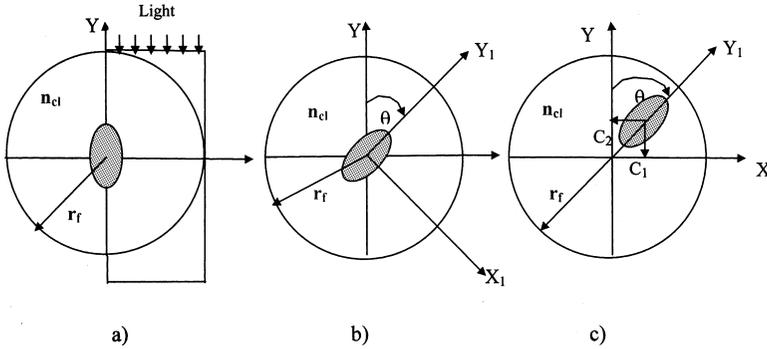
**FIGURE 3** Displays the schematic diagram of the cross sections of different types of the elliptical core optical fibers.
