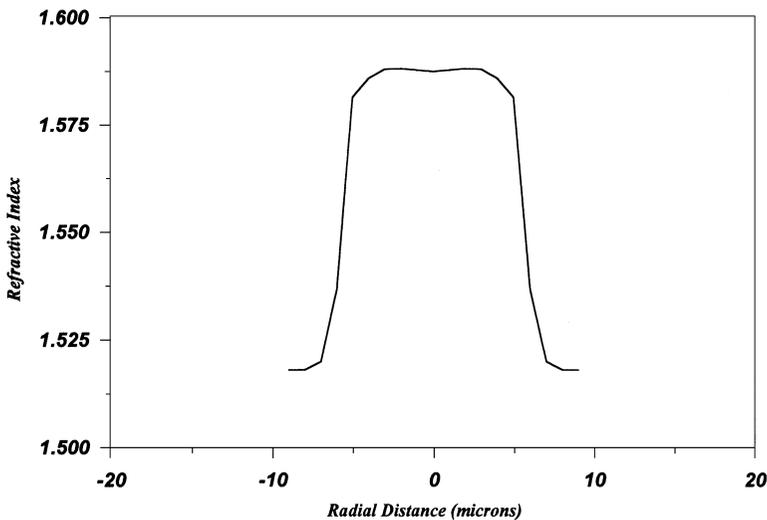
**FIGURE 5** Displays the refractive index profile of the core, which is made an angle  $\theta = 0.0$  deg. with Y-axis, of nine-elliptical core fiber,  $n_L = n_{cl} = 1.518$  and  $\lambda = 632.8$  nm.
