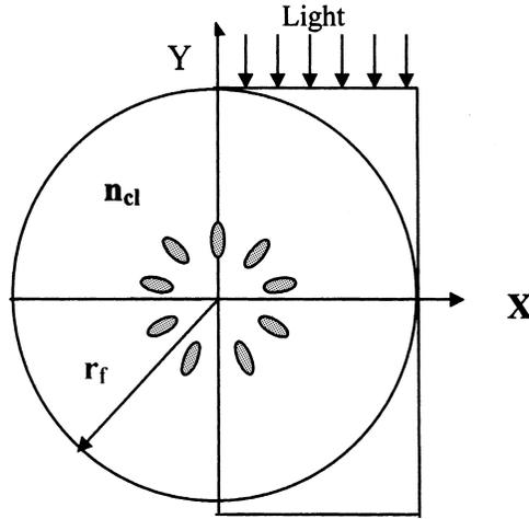
**FIGURE 2** Displays the schematic diagram of the cross section of the identical nine elliptical core optical fiber.
