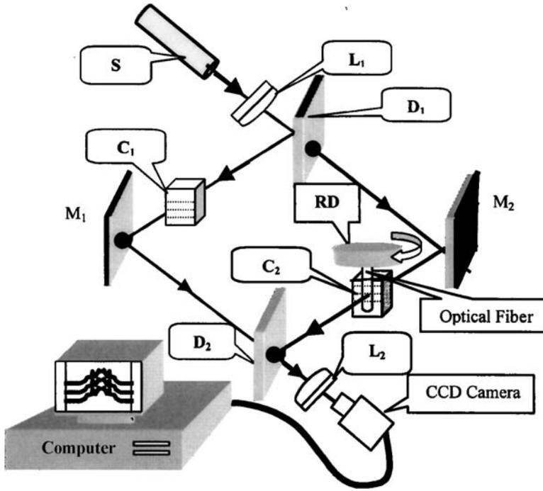
**FIGURE 1** Schematic diagram of computer-aided Mach-Zehnder interferometer; laser beam source **S**, two lenses **L<sub>1</sub>** and **L<sub>2</sub>**, two reflected mirrors **M<sub>1</sub>** and **M<sub>2</sub>**, two beam splitters **D<sub>1</sub>** and **D<sub>2</sub>**, rotating disk **RD**, two liquid quartz cells **C<sub>1</sub>** and **C<sub>2</sub>**, CCD camera, and PC compatible computer.
